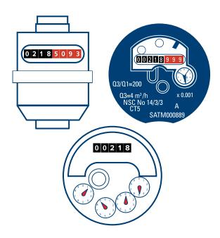
The reading on each of these different meters is 218 kL
