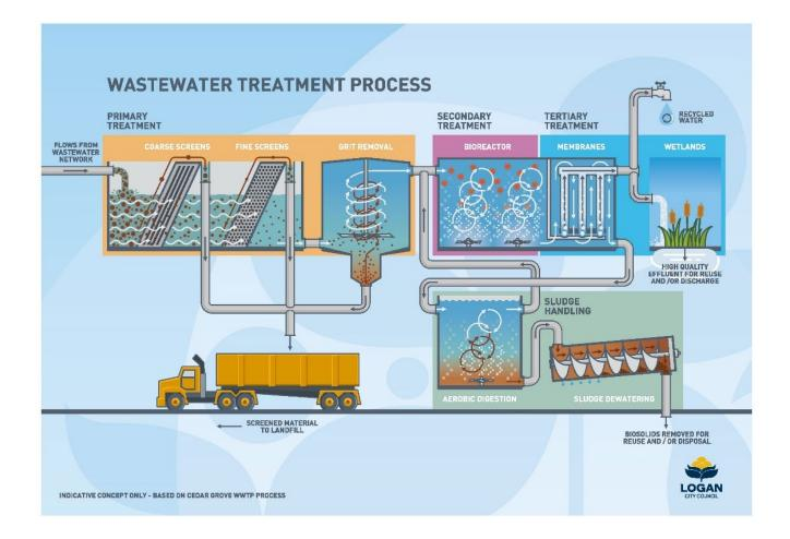
and then at ultimate capacity of about 154,000 people it would be about 25 megalitres per day in dry weather. These volumes would increase during wet weather. For comparison, the Loganholme WWTP currently produces around 44 megalitres per day in dry weather.
